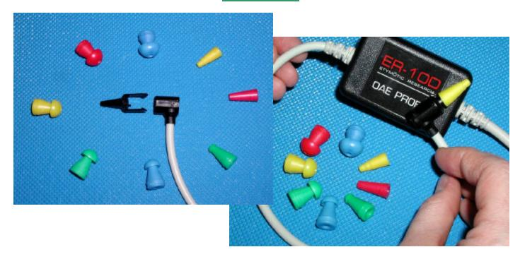
The probe, is very light and can be easily dismantled for cleaning. It is very resistant and insensitive to shocks and tearing, because the transducers are placed into a small box together the preamplifier circuit.
