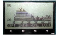
For TEOAE testing the display is switch-able from cross-spectrum data to an automatic evaluation of each tested frequency.
